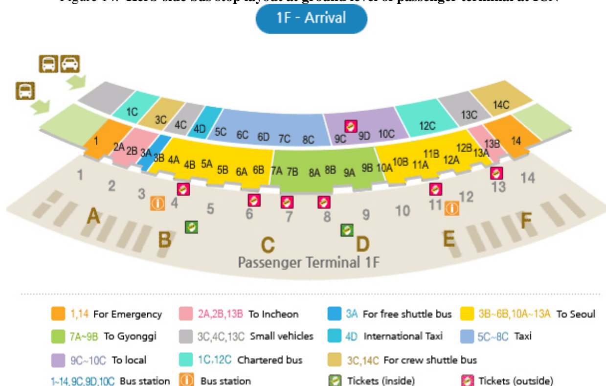
Figure 14. Kerb-side bus stop layout at ground level of passenger terminal at ICN
